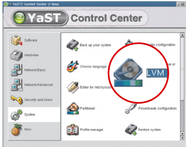
The SuSE Linux Enterprise Server YaST2 installer simplifies adding software to the server. The LVM software RAID manager simplifies creation and management of software RAID partitions.
